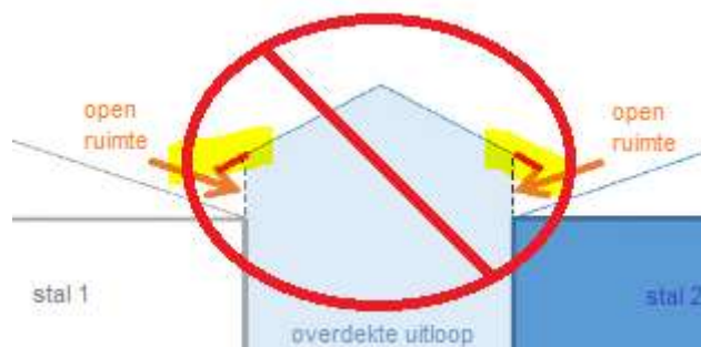
Figure 3. A raised roof of a covered run sandwiched between two buildings must not have a large overhang.
